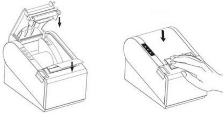
(4) Use the cutter of printer to tear off the extra paper
