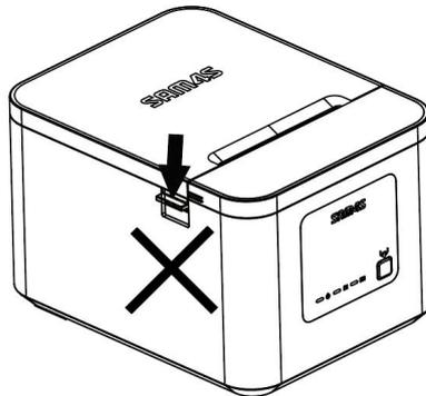
2) Fix the printer by one hand and press either side of the convex bars by the other hand. Push up and open the front cover.
