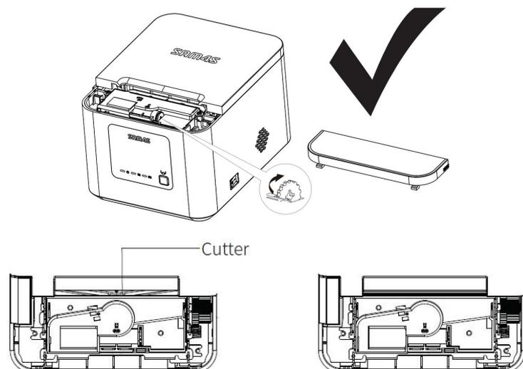
When cutter jam occurs, the auto-cutter blade cannot return to the correct position and it locks in place. In this situation, the roll paper cover does not open even if you pull cover open lever.
